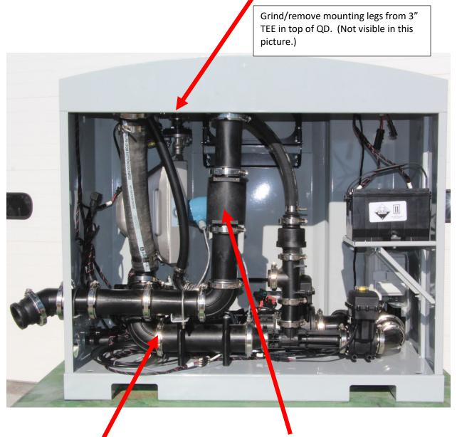
Loosen clamp and rotate to extend 3" wire braid hose gaining approx. 1.5-2" in vertical height.
