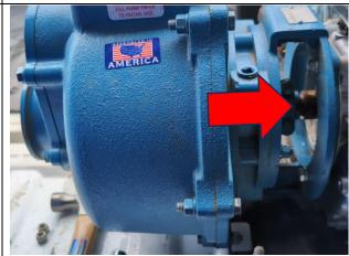
3. Use 9/16" wrench to remove 4 pump mounting bolts from engine assembly. (Save bolts and washers for reassembly)
