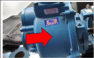
9. The impeller shaft will stop moving and make a solid thud sound when the shaft has been driven as far as it can go. See picture for visual confirmation that impeller shaft is positioned correctly. The round part of the keyway on the pump shaft should be just emerging from the pump.
