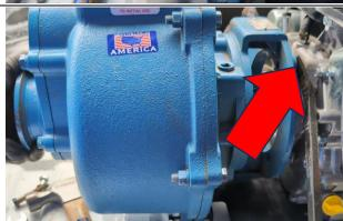
6. Install Shim PN. 400-6679Y2-BK between pump and engine. Reinstall 4 pump mounting bolts to Engine.
