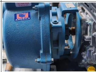
4. Use 9/16" wrench and socket to remove two bolts and nuts attaching the pump to the Engine Mounting Plate.
