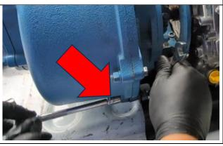
8. Insert dowel into pump inlet. Place dowel on impeller shaft, use hammer to drive impeller towards engine.
