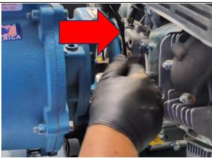
7. Reinstall 2 bolts using 4 stainless steel washers on each bolt between the pump and the engine mounting plate.
