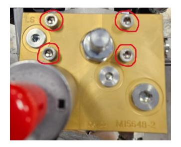
Remove the 4 circled bolts with a ¼" allen wrench Separate PWM valve block from motor and install two new o-rings Reattach PWM valve to motor and reinstall the four bolts.
