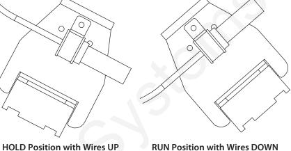
\* The mercury work switch will work with many other controllers. However, the polarity might be reversed from the positions described above. For example, the MT-3405 Series Controllers operate in reverse direction to what is described above.
