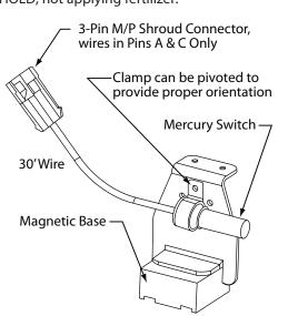
When the mercury in the switch flows against the wires (wires down), the switch will be closed. The Commander will be in RUN, applying fertilizer.
