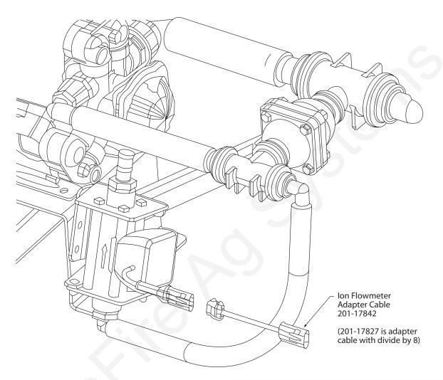
Ion flowmeters are superior to traditional turbine flowmeters in two basic ways. First, they have no moving parts. This translates into no wear items or potential for contaminates to jam a spinning turbine. Second, Ion flowmeters detect the flow of ions which makes them independent of viscosity or density of the fluid measured. They are extremely accurate using standard calibration number. SureFire Ag recommends you perform a catch test to verify the system is properly installed and configured.
