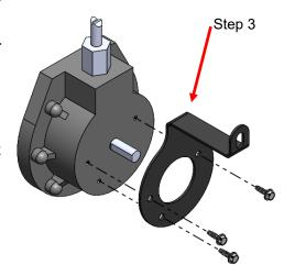
Note: Wire from encoder should be facing down.
