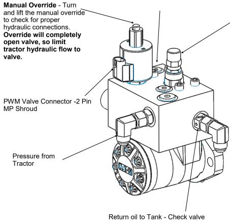
Bypass Valve—Remove the cap to access a bypass needle valve. This valve is shipped from the factory closed. The only case when valve should be open is when running in series with other hydraulic motors.
