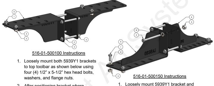
2. After positioning bracket where desired, tighten everything down and Mount Torpedo as shown below.
