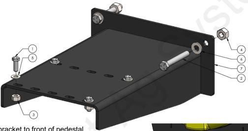
1. Mount bracket to front of pedestal using four (4) 1/2" x 3-1/2" hex head bolts, washers, and flange nuts.
