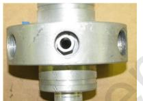
Threaded orifice not installedThreaded orifice installedUse a 5/8" socket wrench to install or remove them when necessary. See picture below.
