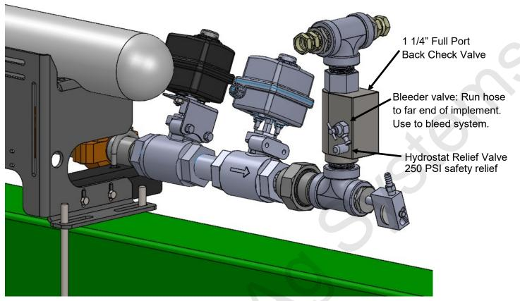
To split the flow to 2 manifolds a Tee is used. If going to 2 manifolds with electric section valves 1" high pressure hose is used (equal length to each manifold).
