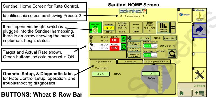
The wheat button takes you to the Multi-Product RUN SCREEN (below). This button appears on the right side of the screen. Pressing it puts the Operate > Setup > Diagnostic view on the bottom third of the with
