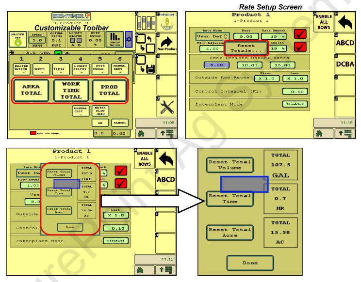
Push any of the **Reset** buttons to reset that total to 0. To return without changing any of the totals, press **Done.**
