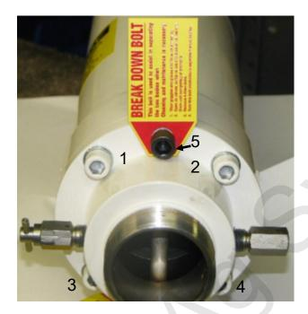
2. Replace both inner o-ring dump seals and body o-ring seal. Repair kit part number 153-01-A-SF-RK. Lubercate the O-rings before installing them in the Toppedo tube and torque the bolt to 35 ft-lbs.
