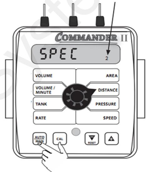
**NOTE: The above procedure will load all default values in the Commander II. It must be done before standard calibration.** For example, if you entered your implement width, then did the quick setup above, the Commander II would default back to 240 inches.
