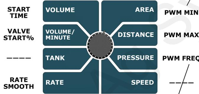
**RATE SMOOTHING:** This value is used to help the system lock on to the target if all system parameters seem to be functioning appropriately.
