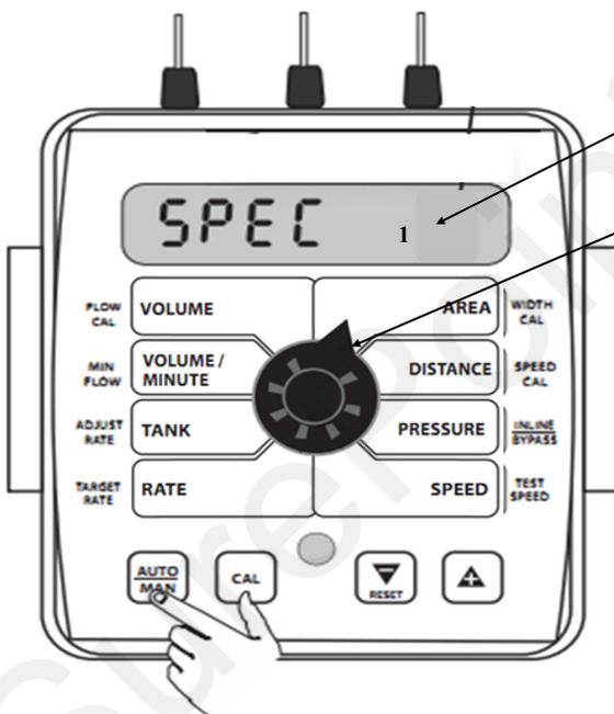
This number tells you which special CAL screen you are on. Pressing the CAL button will change this number. Quick Setup is on Page 1, with dial turned to AREA.
