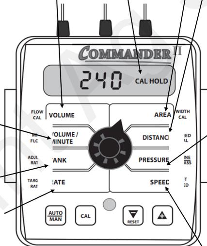
**CONTROL SPEED:** Typically -4 for PumpRight Hydraulic Pumps.
