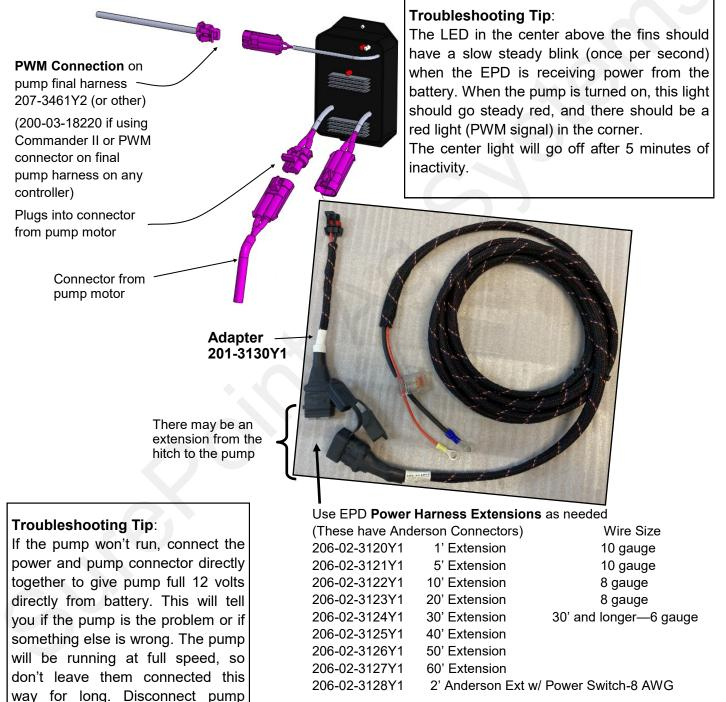
SurePoint recommends a single long extension harness as multiple connectors will reduce voltage, increase current and hurt performance of your electric pump system.
