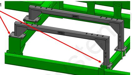
3. Finally, install tank in the saddles and fasten the tank strap mounting brackets, and tank straps. Check for clearance.
