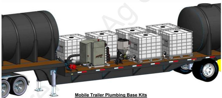
These kits are used to plumb a trailer such that the QuickDraw can be used to fill tanks individually, and use carrier blending to pull from the desired tank during operation.
