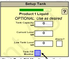
Check **Tank Fill Monitor** box if using a fill flowmeter (not used very often). Then enter **Tank Fill Flowmeter Cal.**
