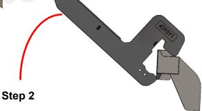
3. Use the 425-4297Y1 and 425-4298Y1 pinch plates to tighten the mounting bracket to the weight bar. Fasten using the 1/2" x 1-1/2" hex head bolts and 1/2" nuts. The tank mounting bracket should be securely fastened so that there is no movement.
