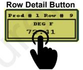
From the HOME screen, touching the row detail button will display the row detail page. The user can toggle through the rows by touching the buttons. The user can also pause the Auto Scrolling feature pressing the Pause Scan button.
