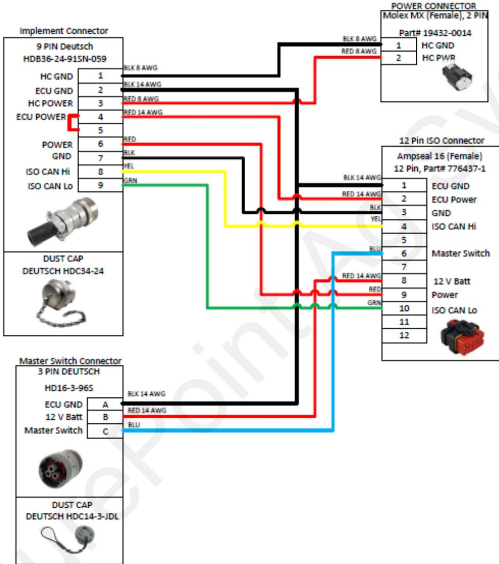
Include and Connect the CAN BUS Terminator Harness
