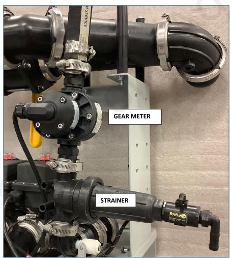
The Gear Meter system also comes with a paddle flow switch plumbed into the line before the strainer. This flow switch guarantees that product is flowing when the meter is spinning. The meter can turn from the venturi suction even if no product is flowing. With the flow switch, the controller will not read flow if the meter is spinning without any liquid flow. The flow sensor is displayed on the Manual Operation screen.
