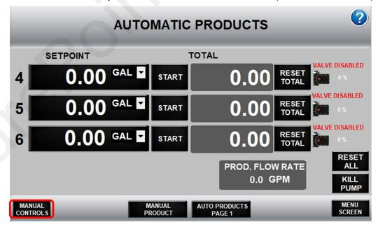
MANUAL CONTROLS brings up the Manual Operation and Debugging Screen.
