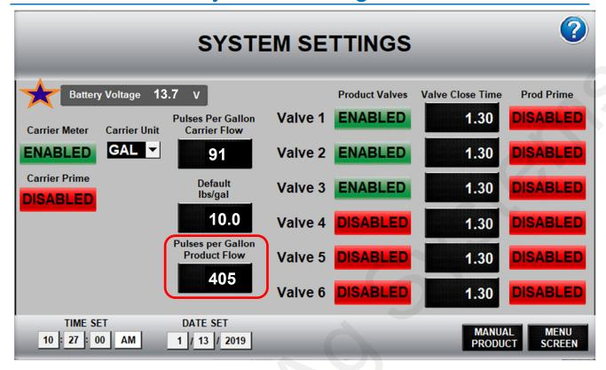
If a carrier flowmeter is installed, set **Carrier Meter** to **ENABLED**. Adjust Pulses per Gallon as needed, default pulses per gallon for water is 91. This may need calibrated when using fertilizer as a carrier or if the batch is consistently over or under the target.
