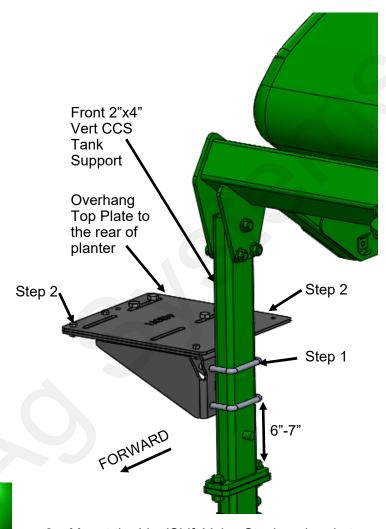
Mount the LiquiShift Valve Stack on bracket as shown to the left using the supplied 1/2" Hardware. Make sure the valve stack is mounted to the rear of the support bracket. If this is not the case, collision when folding planter could become an issue.
