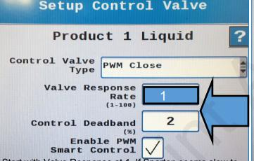
Start with Valve Response at 1. If Spartan seems slow to adjust, increase this number by 1 at a time. If system won't lock on, change Advanced Tuning > P = 5, S = 0.9. Press and hold the System Settings tab for 10 seconds to bring up the Advanced Tuning button.
