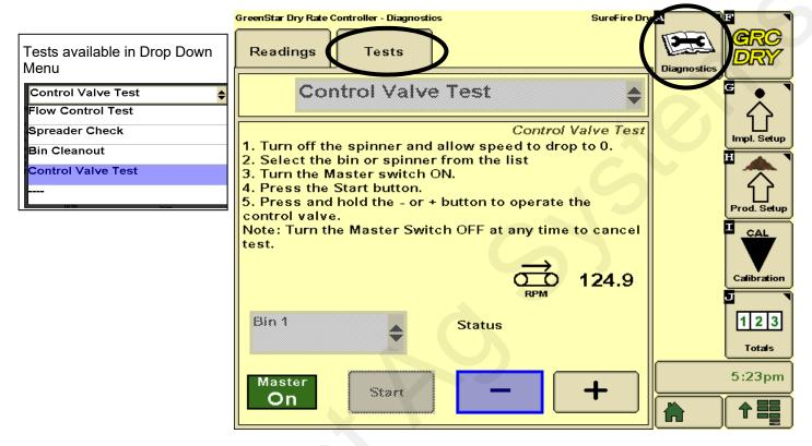
It is not always necessary to run this test. It may or may not give useful results. If the system responded well on the previous Control Valve Test
