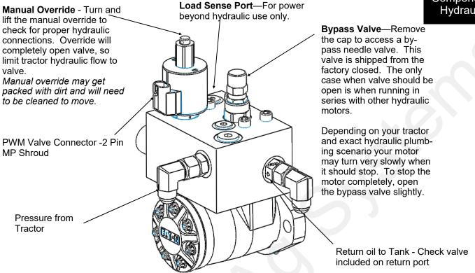
Port Sizes: -8 SAE O-Ring (Load Sense is -6 SAE O-Ring)
