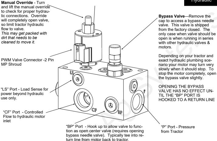
Pressure and Controlled Flow Port Sizes: -12 SAE O-Ring
