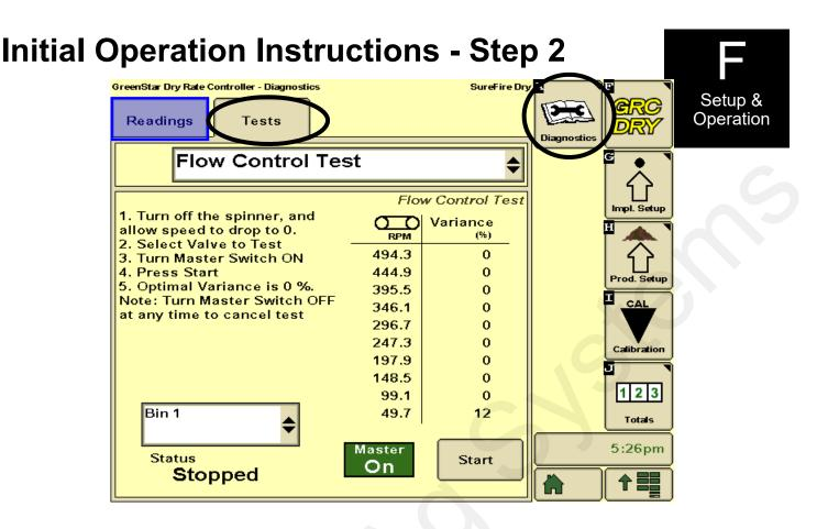
This test may not be necessary to run, but it will help you see how the controller controls the system. The Variance numbers may not be especially helpful. If the Control Valve test worked OK, go on to the CFR Calibration.
