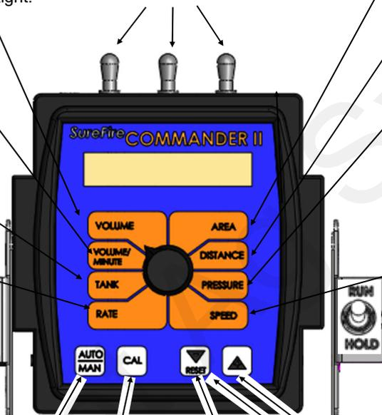
**CAL:** This key is used to enter & exit calibration (CAL) mode.
