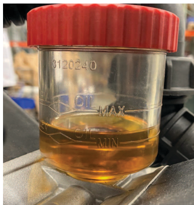
Figure 14. PumpRight Oil Fill & Sight Glass
