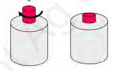
**Preseason -** Clean the dirt out of the stem for the red knob so the red knob can be moved by hand. Be sure to lock it in the down position before operating
