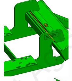
2. Set the 425-3995Y1-GN bracket on the front weight mount bar. This is best achieved by tipping the front, aligning to the center post until the top of the bracket falls behind the lip and then lowering the front of the bracket.
