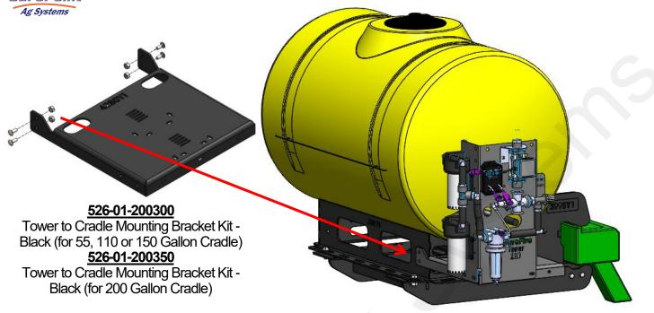
2. Mount the tower mounting bracket to the cradle using (4) provided 3/8" carriage bolts and flange nuts.
