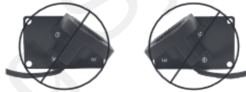
Incorrect mounting positions
