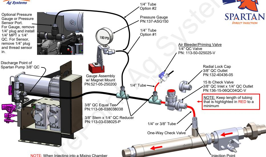
NOTE: When Injecting into a Mixing Chamber or Main Product Line with the Spartan Pump, you must use a One-Way Check Valve at the Injection Point to prevent back flow to the Spartan Pump.
