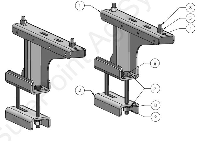
SurePoint Accelerator (55, 110 and 155 gallon) or Catalyst™ (55 and 110 Gallon) tanks can be mounted above and offset from a toolbar using this z-mount bracket.
