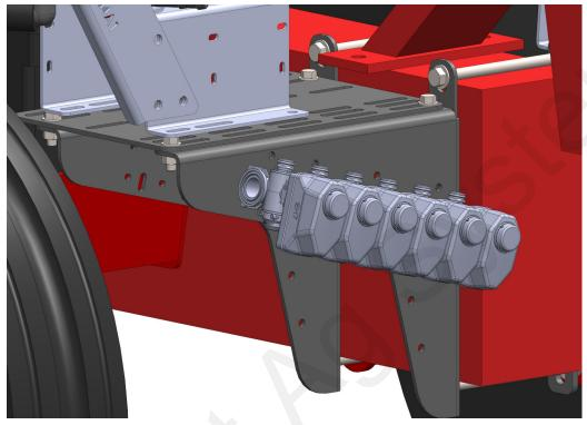
Up to three (3) Banjo Section Valves may be u-bolted to the side of the pump support bracket using the larger bolt hole and slotted hole in the center as illustrated below.
