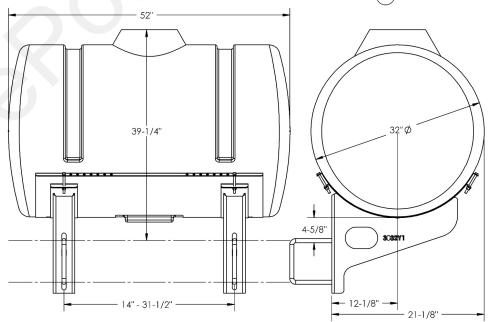
396-3090Y1 - Offset Saddle Mount 23" and 32" Diameter Tanks
