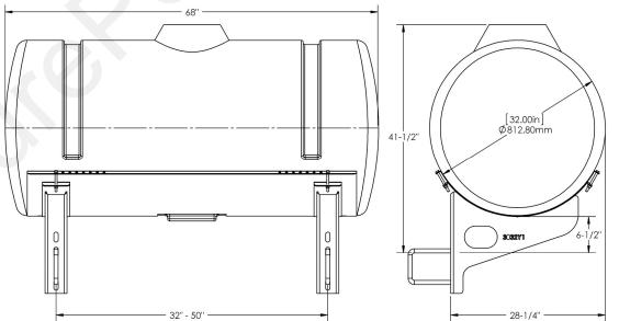
396-3090Y1 - Offset Saddle Mount 23" and 32" Diameter Tanks
