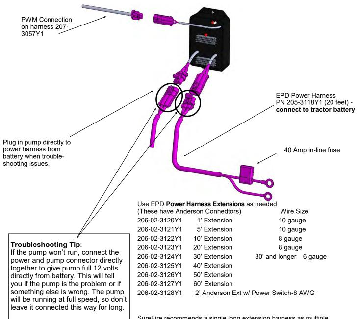
SureFire recommends a single long extension harness as multiple connectors will reduce voltage, increase current and hurt performance of your electric pump system.
