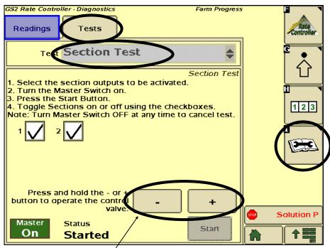
Go to Step 2 on the next page when you can increase and decrease the GPM reading using the + and - buttons.
