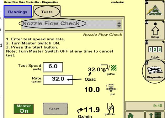
8. You can use this procedure with product (instead of water) to verify your minimum pressure is at least 10 psi (to ensure all check valves open). Also check the maximum speed and rate to make sure pressure is under 50 psi.
