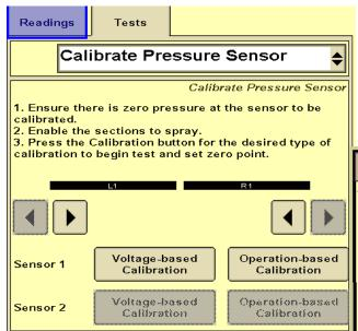
Tip: If the system has been running, there may be pressure in the system due to the check valves. In that case, simply unplug the sensor while this setup is being done so it will calibrate the zero point correctly.
