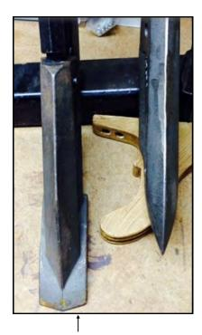
The knife on the left is for notill conditions. On the right is a less aggressive point for tilled soil.
