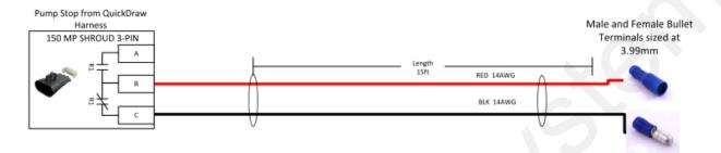
Figure 2: 208-05-2633Y1 Pump Stop Harness (Grounded Coil)
