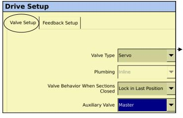
Set the Valve Setup as shown.
