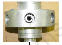
Threaded orifice installed
