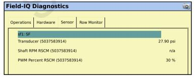
The **Sensor** tab provides information on the Pressure Sensor.
