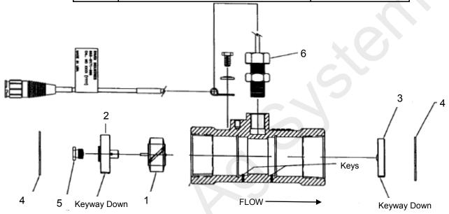
**RFM 60S Flowmeter Maintenance and Adjustment Procedure**
