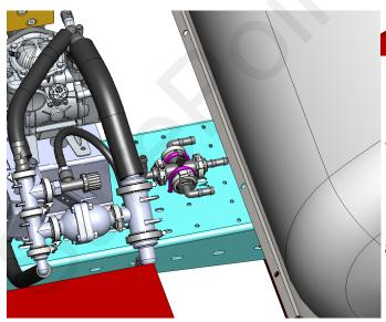
7. Use PN: 520-00-045000 assembled like picture to the left. Run 3/4" hose from assembly to stainless steel manifolds already mounted in previous steps. OPTIONAL: Section valves may replace this assembly.
