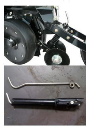
This tube does not fit on 2012 model Case planters or newer. For tubes that fit the 2012 & newer Case planters see part # TT-10012.
