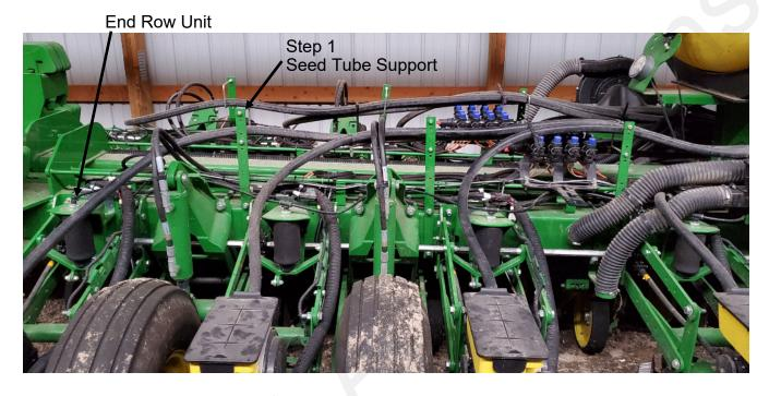
2. Install both base mount brackets (420-4452Y1-BK) with supplied 3/4" U-bolts (380-1060) as shown below. Make sure the Gusset is facing forward on the planter, see Figure 1 below.
