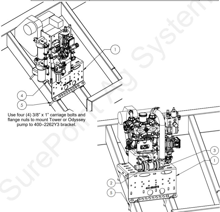
Use four (4) 1/2" x 1" hex head bolts and flange nuts to mount PumpRight pump unit to 400–2262Y3 bracket.
