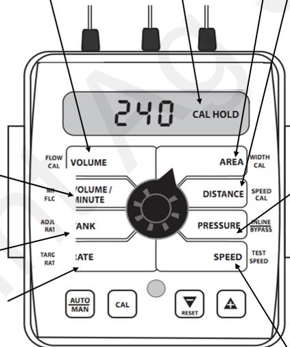
**DO THIS - WIDTH CAL:** Enter the width of each fertilizer or chemical section of your implement. For a single section system, set Section One to the full implement width in inches. For example, for an 8 row 30" implement, set Section One to 240 inches. To set the section widths the Run/Hold Switch has to be in Run and the Section Switch must be ON. If using a single section implement, set Section 2 and 3 to ZERO.
