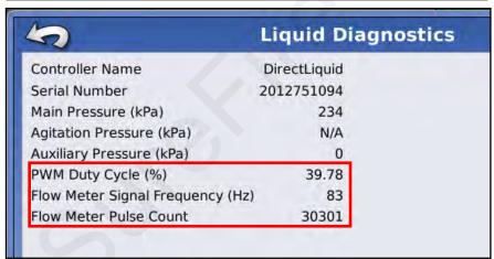
**PWM Duty Cycle** is an indication of how fast the controller is telling the pump to run. The controller adjusts the PWM Duty Cycle to speed the pump up or to slow it down.
