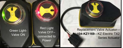
If valve indicator stays GREEN all the time or if valve indicator is not in full ON or full OFF position, replace actuator. Pull gray pin to remove actuator from valve.
