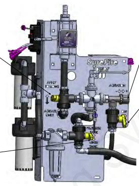
Agitation Adjust Valve: RECIRCULATION KNOB: This valve adjusts how much flow returns to the tank while working in the field. Normally closed. If needed, start with a quarter turn.
