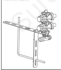
The check valve is mounted over the top of the bar. The supply line would run above and behind the bar. The short bracket is placed in the notch to mount the check valve closer to the bar.
