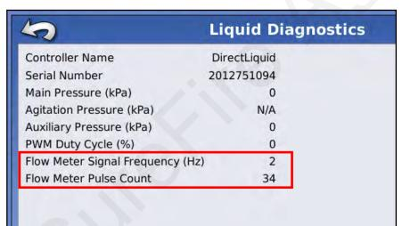
During Flowmeter Tap Test a small number should register on the Flow Meter Signal Frequency and the Flow Meter Pulse Count should increase.
