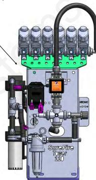
The Tower 110 can have up to 6 section valves mounted directly to the top of it with this bracket.
