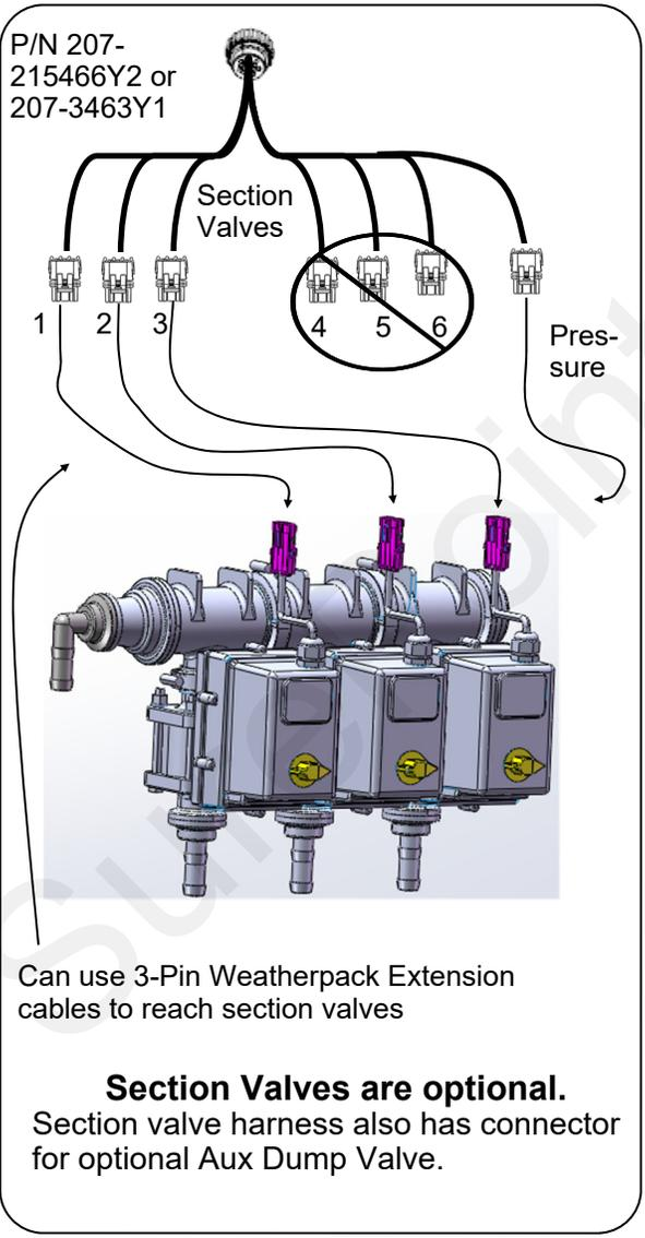
Each harness has connectors for Pressure 1 (Main) and Pressure 2 (Aux).
