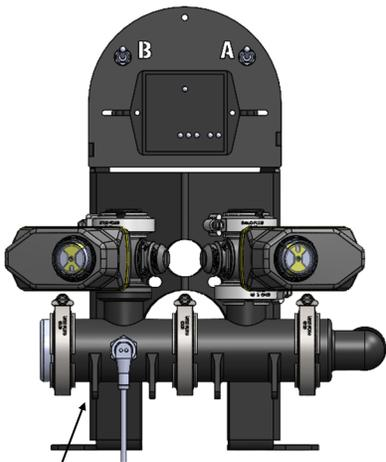
Pressure Sensor for LiquiShift is mounted at the base of the valve stack. The same sensor is used for LiquiShift and displayed on the Ag Leader display.
