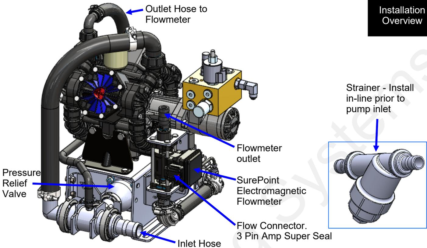
**Inlet:** The PR17 and PR30 PumpRight are shipped with a 1 1/2" inlet hose barb. Attach this to the hose from your supply tank and strainer. A 1 1/2" 90 degree hose barb is included and can be substituted.
