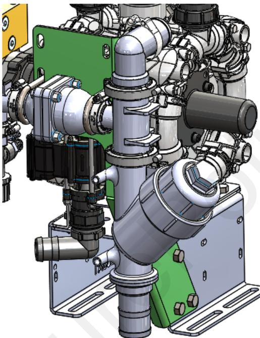
**Inlet:** The PR40 and D250 PumpRight are shipped with a 2" inlet hose barb. Attach this to the hose from your supply tank and strainer. A 2" 90 degree hose barb is included and can be substituted.
