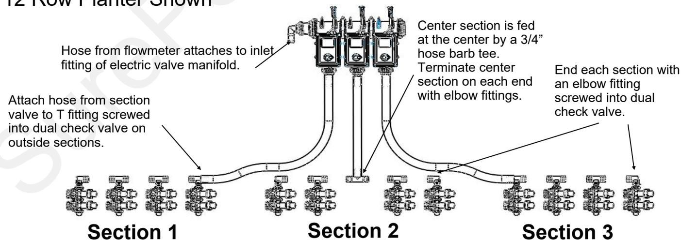
For a 2 section plumbing system, omit the center section and plumb similar to the outside 2 sections.
