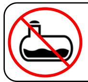
SurePoint Ag Systems <u>does not</u> recommend transporting your implement with full fertilizer tanks. Doing so can result in damage to brackets and implement.
