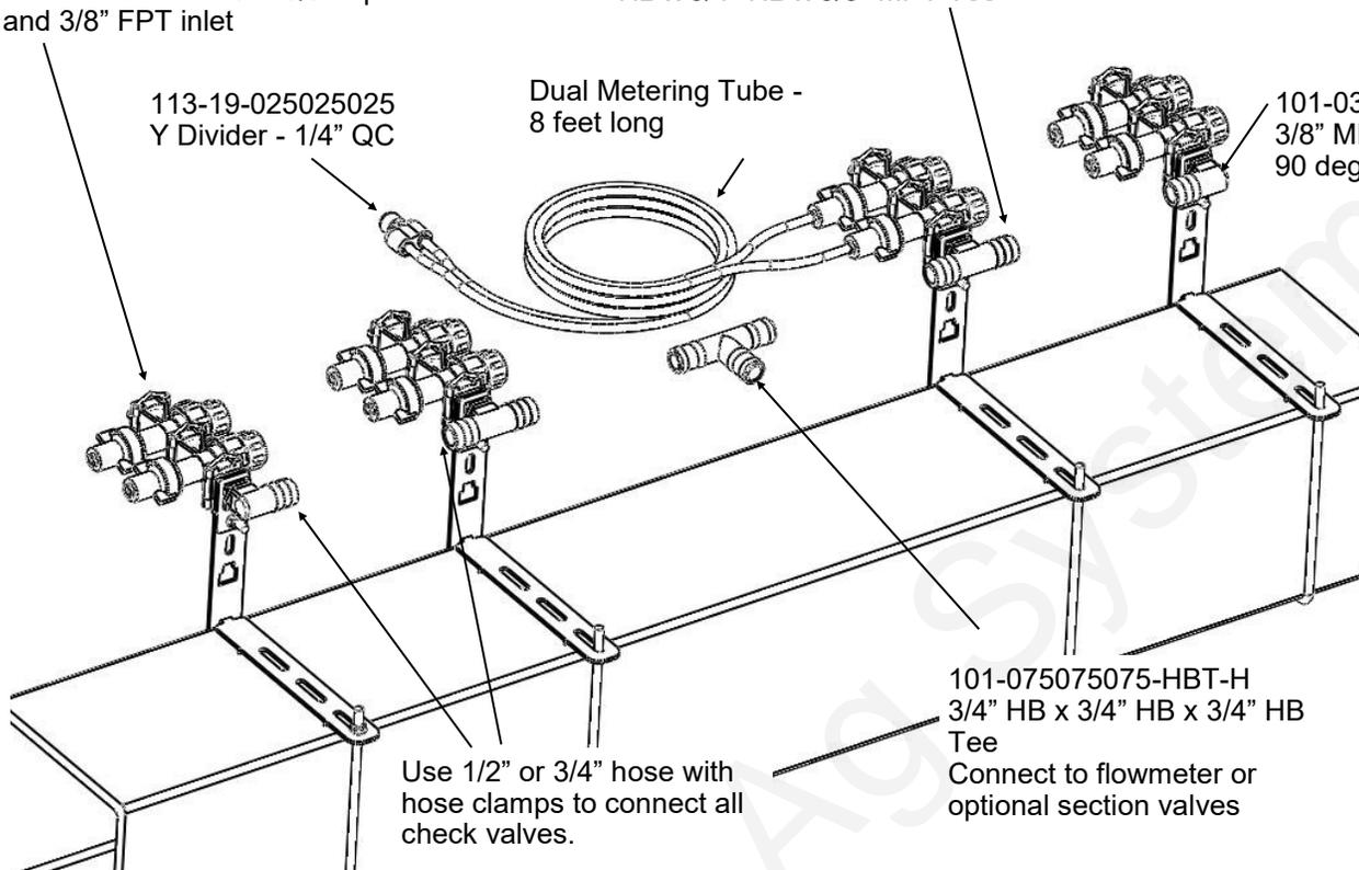
This is a general diagram showing the dual check valve assembly mounted on a planter toolbar. The check valve and bracket are very flexible in their mounting. The check valve can mount behind, directly over, or in front of the toolbar. The check valve can be put in the bracket facing up & down or sideways (shown). In addition the steel bracket could be rotated 90 degrees and clamp around the bar. The multiple slots in the bracket are used to mount to any tube 7x7 inches or smaller.
