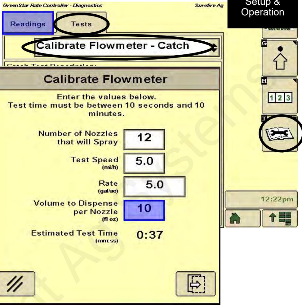
With SurePoint Electromagnetic flowmeters, most times the sample volume is correct. In that case, just enter the same sample size you did in #5 above to leave the calibration value unchanged. If the sample volume differs from what is expected, recheck the calibration settings. Do not change the calibration value if there is a small difference in the sample volume. It takes a fairly large sample from several rows to get a number that is accurate enough to change the default Flowmeter Calibration.
