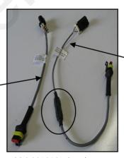
With the 0.13 – 2.6 and 0.3 – 5 GPM models, the 'Divide by 8' adapter harness MUST be used. It is PN 201-17827. It must be used because the GS2 controller limits the maximum calibration number. The 'divide by module' is circled.
