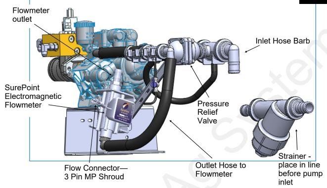
**Inlet:** The D70 and D115 PumpRight is shipped with a 1 1/2" inlet hose barb. Attach this to the hose from your supply tank and strainer. A 1 1/2" 90 degree hose barb is included and can be substituted.
