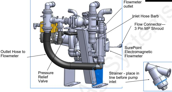
**Inlet:** The D160 and D250 PumpRight is shipped with a 2" inlet hose barb. Attach this to the hose from your supply tank and strainer. A 2" 90 degree hose barb is included and can be substituted.
