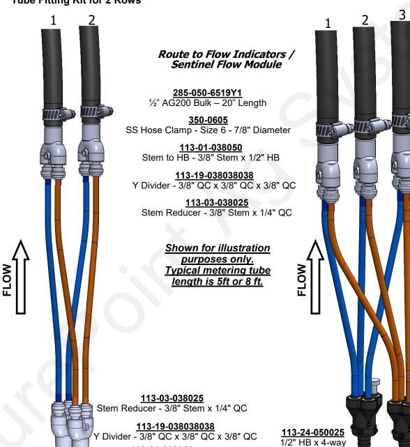
Plumb to"A" Valves Larger DIA Metering Tubes
