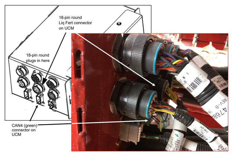
Main Adapter Harness 213-05-3873Y3 plugs into the 18-pin round connector and the 12-pin CAN4 (green) on the UCM on the planter. Unplug the Case connectors in these positions, plug in the SureFire harness, then plug the Case connectors into the SureFire harness. Then plug the Sentinel (or RCM) adapter harness into the ISO and POWER connectors on the 3873 harness.
