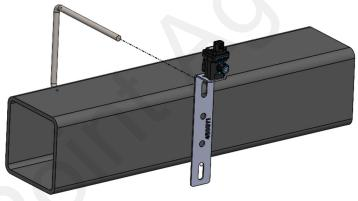
3. Route 3/8" OD tubing or 3/8" OD hose from the flow indicator or Sentinel Flowmeter Module to the row unit. Use the provided 3/8" Stem x 3/8" QC elbow as needed to make a sharp turn into the valve.
