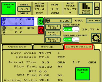
**Diagnostic:** (PWM) **Duty Cycle** shows the PWM signal sent from the controller to control the pump. On a hydraulic system, this needs to be around 30% before the pump will run. 40%- 50% is a typical operating range. On a normal pass this should be fairly stable (± 2%). The Duty Cycle will adjust for speed, rate changes or width changes (sections going on and off).
