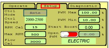
**Ctrl Speed:** Decrease if pump surges or oscillates back and forth above and below the rate. Increase if pump is slow to adjust.
