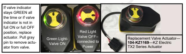
*This is a 3-way valve*. If product will not flow when valve is ON, either move the outlet hose to the other outlet port, or remove actuator and rotate valve ball 180°, and replace actuator. Product should flow through the port closest to the Indicator light when the valve is open (green).
