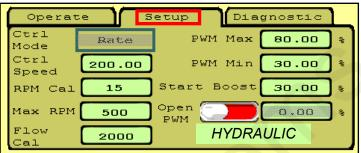
**Flow Cal** can be adjusted slightly if an accurate catch test or field verification indicates it should. Increase Flow Cal if more product is needed. Decrease flow cal if less product is needed.
