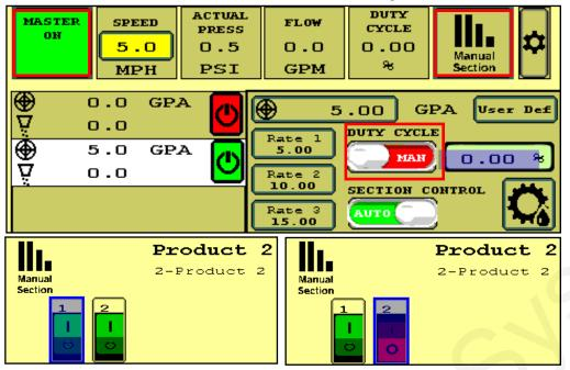
To operate the Section Valves manually, press **Manual Section**, then press any section button to turn the valve off/on.
