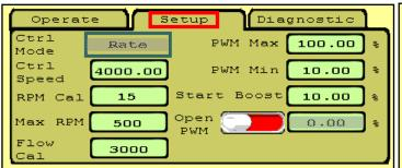
**Ctrl Speed:** Decrease if pump surges or oscillates back and forth above and below the rate. Increase if pump is slow to adjust.
