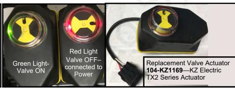
This is a 3-way valve. If product will not flow when valve is ON, either move the outlet hose to the other port, or remove actuator and rotate valve ball 180°, and replace actuator.
