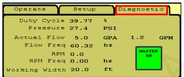
**Diagnostic Tip:** Note the relationship between Duty Cycle (%), Pressure, Flow (GPM), and RPM (hydraulic pump). If Duty Cycle and RPM increase above what Is normal for a given flow, there could be a restriction on the inlet side of the pump. This could be a plugged strainer or a strainer that gets gelled over, especially with cold fertilizer.
