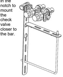
Example 3. Use the long bracket on the front of a 3x7 bar (vacuum tube on some planters). Mount the check valve hanging forward of the bar. The supply line will run directly over the bar. The excess bolt and bracket Short length **Bracket** can be cut off.
