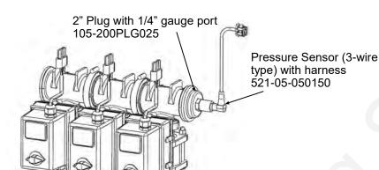
0 to 5 v - 100 PSI Pressure Calibration: 50 mv/psi
