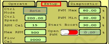
**Flow Cal** can be adjusted slightly if an accurate catch test or field verification indicates it should. Increase Flow Cal if more product is needed. Decrease flow cal if less product is needed.
