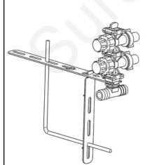
Example 2. Use the long bracket on the rear of a bar. The check valve is mounted over the top of the bar. The supply line would run above and behind the bar. The short bracket is placed in the notch to mount the
