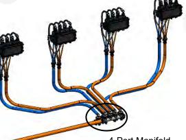
4-Port Manifold mounted on each wing
