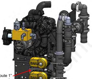
Gen 3 LiquiShift A/B Valve Bolt-On Kit for PR40/D250 (MEVX) - 3rd Party Control <u>Kit: 522-03-100250</u>
