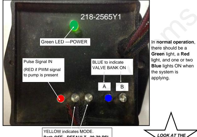
YELLOW indicates MODE. **Both OFF—DEFAULT –20-70 PSI** Left ON—20-80 PSI Right ON—20-60 PSI Both ON—15-40 PSI (Tower Demo)
