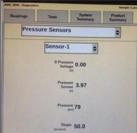
*Diagnostics > Readings > Pressure Sensors* will show this voltage and pressure if the harnessing is good.
