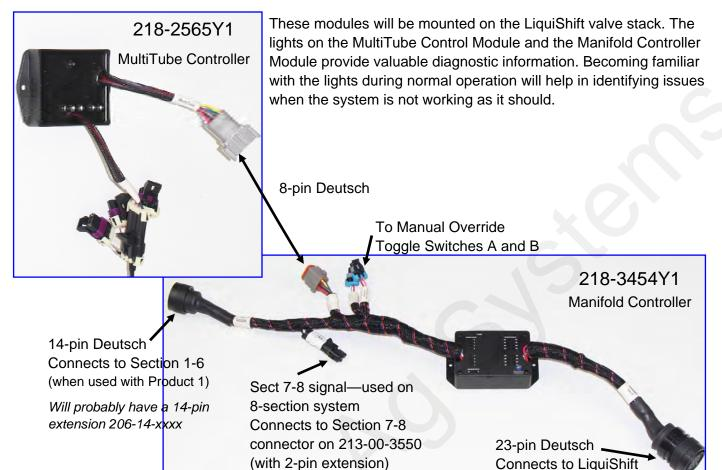
The **MultiTube Controller** (218-2565Y1) is mounted on the back of the LiquiShift tower, behind the **Section Manifold Control Module** (218-3454Y1).
