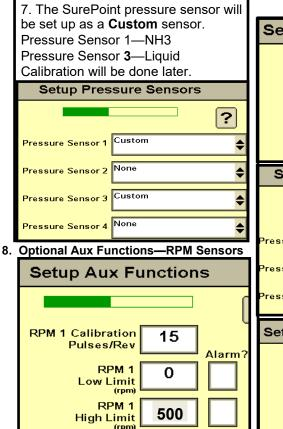
The SurePoint hydraulic pump with an **RPM Sensor is 15 pulses/rev** as shown. If monitoring something else, enter the pulses/rev for that encoder or sensor.)
