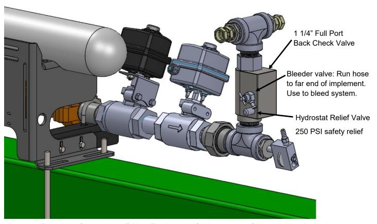
To split the flow to 2 manifolds a Tee is used. If going to 2 manifolds with electric section valves 1" high pressure hose is used (equal length to each manifold).
