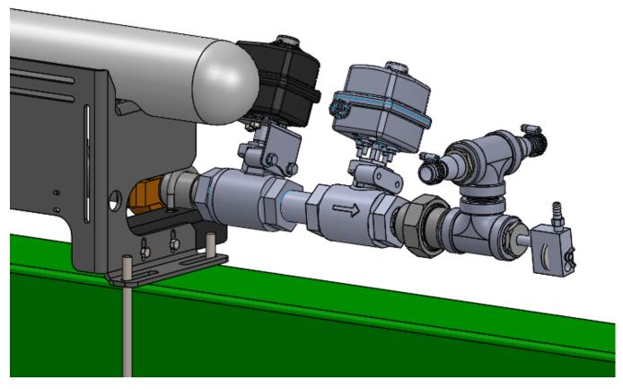
To split the flow to 2 manifolds a Tee is used. If going to 2 manifolds with no electric section valves 1" reinforced EVA hose is used (equal length to each manifold).
